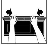
bottom until it snaps into place. Replace the mounting screws.
